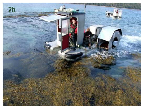
Figure 2: Harvesting methods for a) Laminaria hyperborea , the seaweed trawl and for b) Ascophyllum nodosum the paddlewheel cutter. Photos: a) FMC Biopolymer AS, b) Sander Andersen
